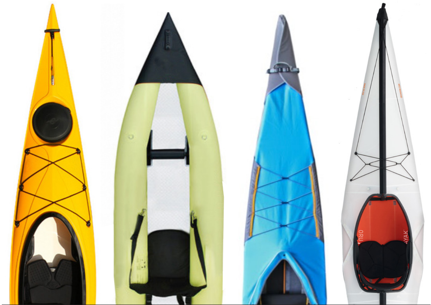
Rigid Inflatable Skin-on-frame Oru Kayak
